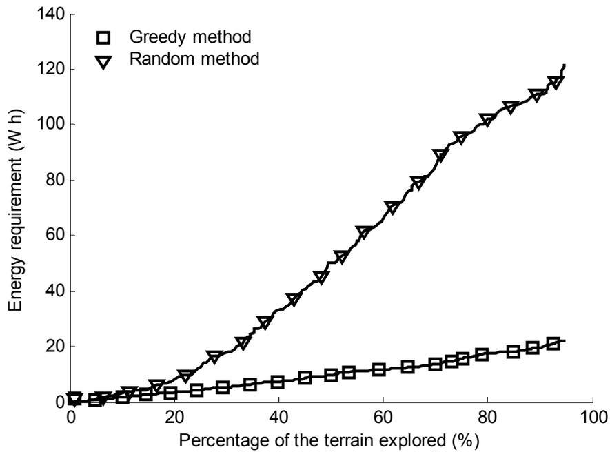
Figure 5. Result of the autonomous construction of an agricultural field map: energy requirement of the exploration as a function of fraction of explored terrain.
