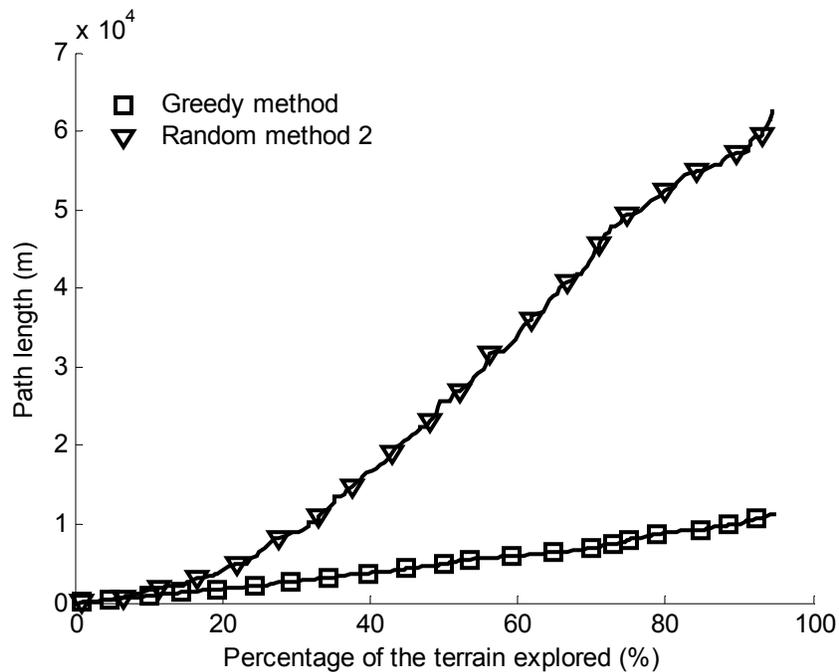
Figure 6. Result of the autonomous construction of an agricultural field map: path length traveled by the robot as a function of fraction of explored terrain.
