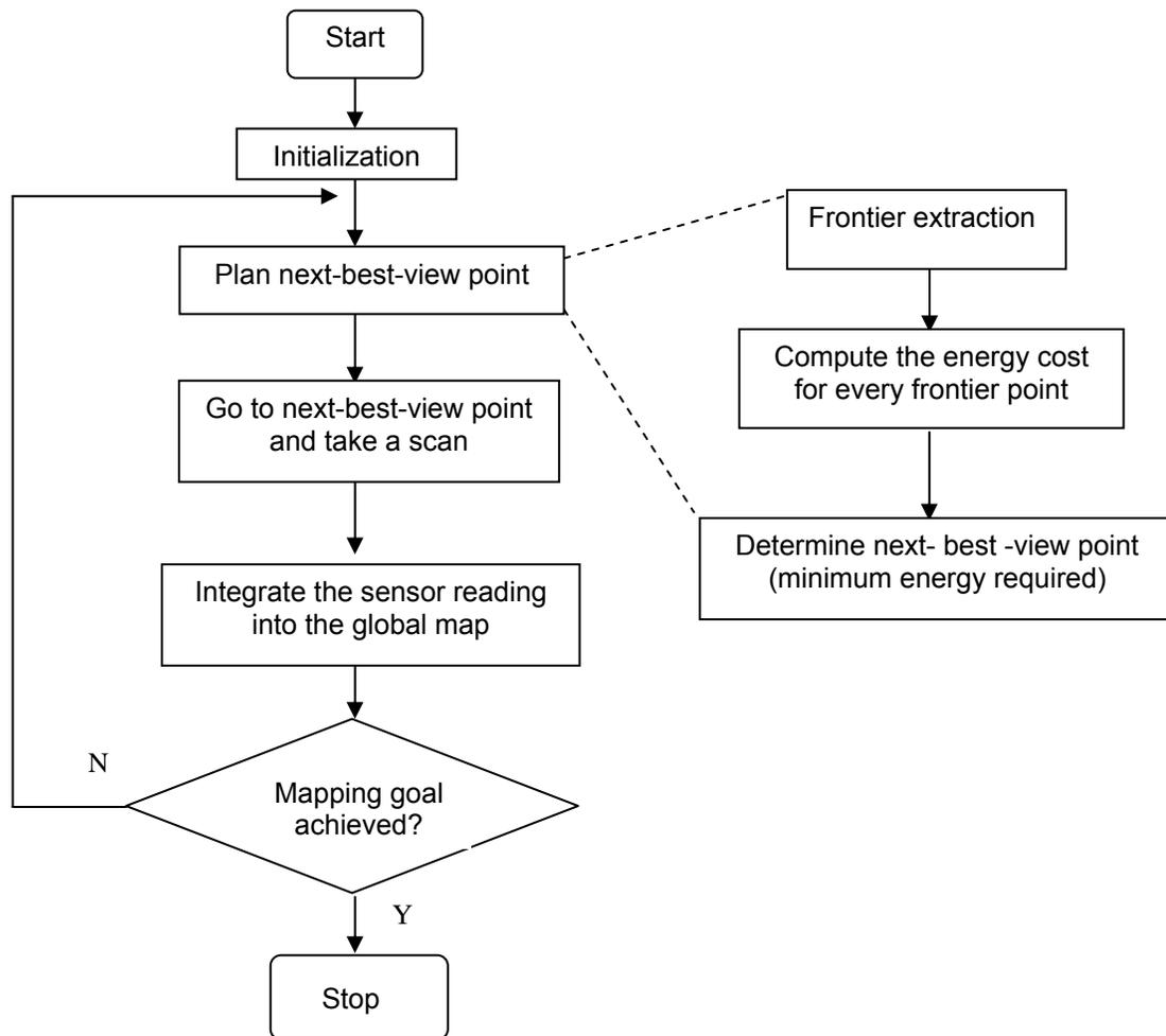
Figure 3. Next-best-view algorithm flow diagram.
