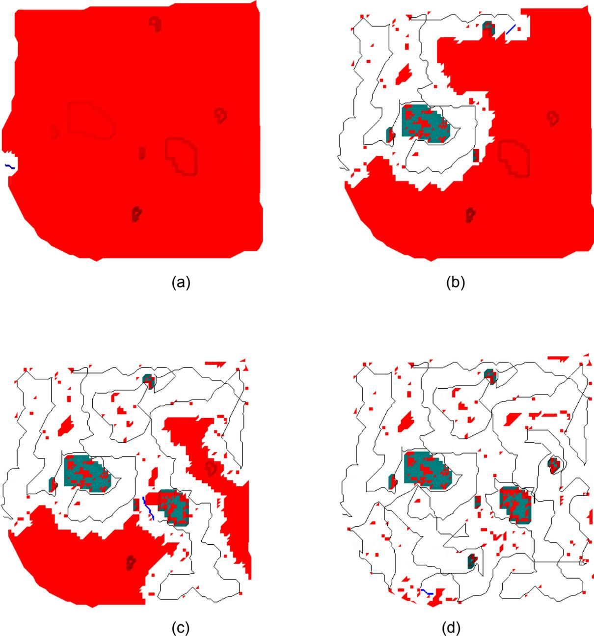
Figure 4. The traveled path (black lines) and updated map (white parts are explored terrain) are plotted at selected iteration times: (a) initialization; (b) after 70 iterations; (c) after 140 iterations; (d) after 208 iterations.
