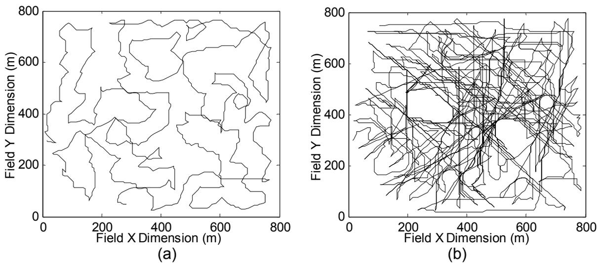
Figure 8. Trajectory generated in the simulation: (a) greedy method; (b) random method.
