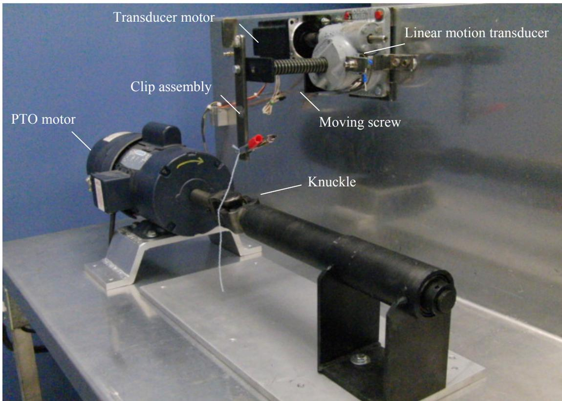
Figure 1. Experimental apparatus used to expose a hanging strand of yarn to a rotating PTO knuckle.
