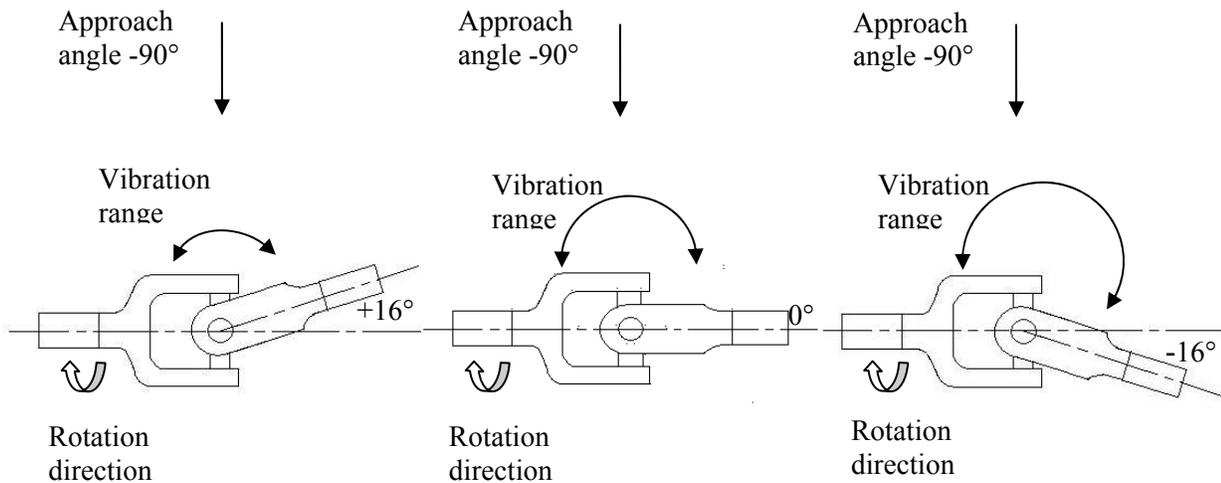
Figure 4. Vibration ranges at the spinning knuckle with different joint angles (Top view)
