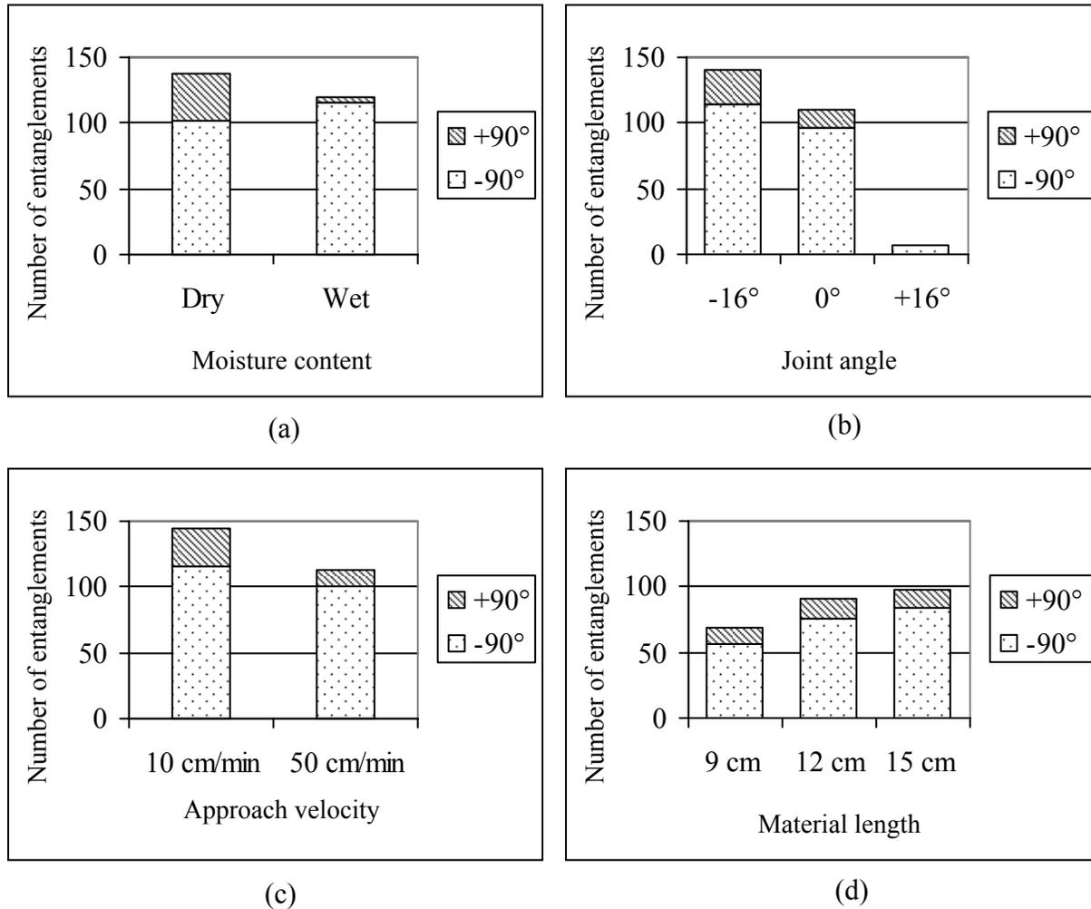
Figure 2. Distribution of number of entanglements at +90° and -90° approach angles in each comparison group: (a) Material moisture content; (b) Joint angle; (c) Approach velocity; (d) Material length
