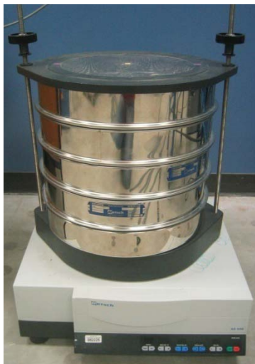
Fig. 5. Retsch sieve shaker: screens and collecting pan, used for sizing.
