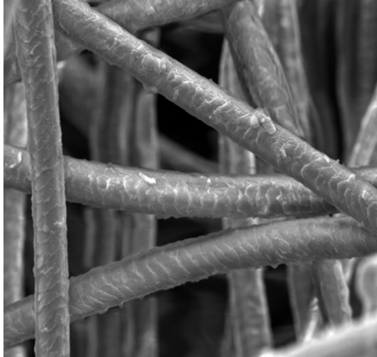
Figure 5 An ESEM micrograph of a mass of alpaca wool (Magnification: 1000x, Working distance: 17.1mm)
