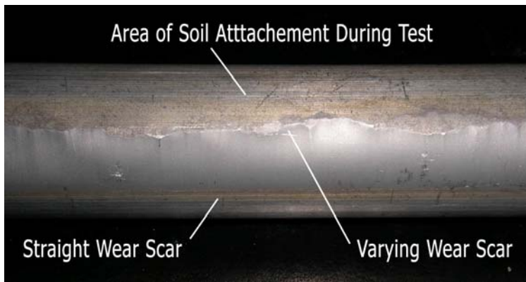
Figure 5. Variance in soil attachment creates an uneven wear edge as seen from the bottom of the specimen (90 degrees).
