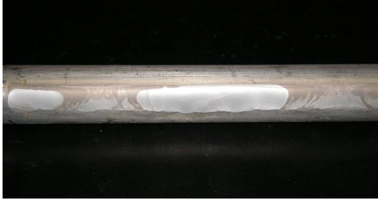
Figure 6. Wear scar layering caused by differences in soil attachment over a set of runs.
