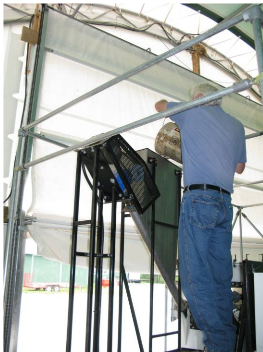
Figure 3 Liquefied inputs being added to feed auger
