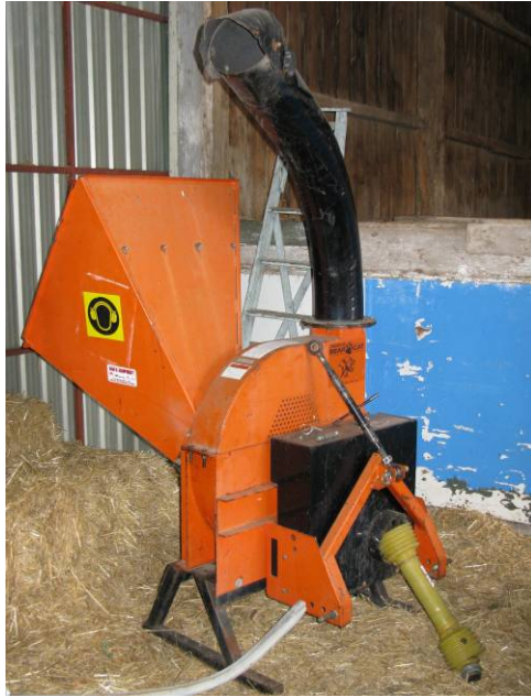
Figure 2 Wood chipper used to process sugar beets prior to digestion
