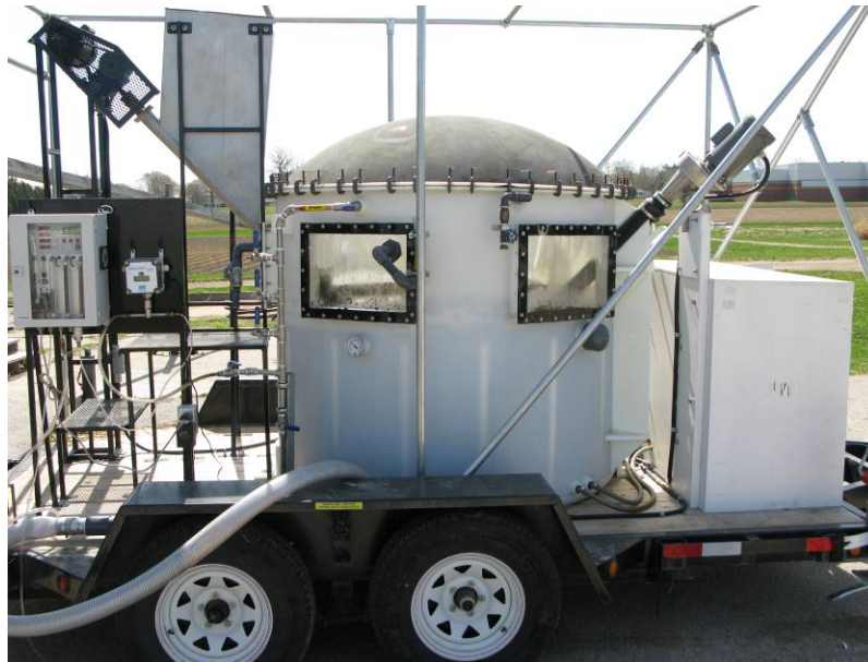
Figure 1 - Portable 2.2 m 3 anaerobic digester
