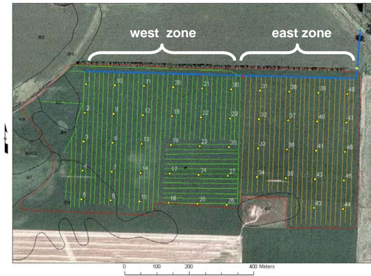
Figure 1. Drainage system layout showing east, controlled drainage, and west, conventional free-drainage zones and 48 geo-referenced sampling locations.
