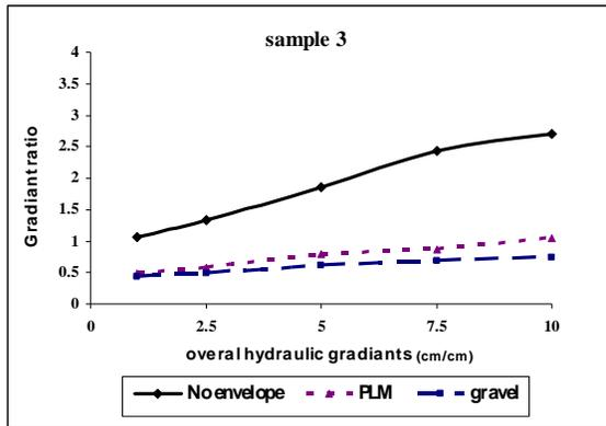
Figure 6. The variations of the gradient ratio index vs. the system hydraulic gradient.
