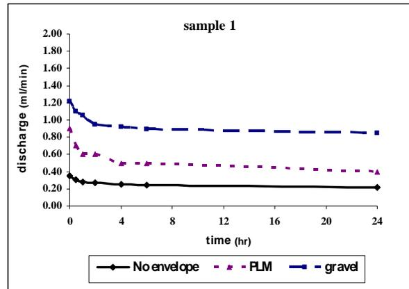
Figure 4. The outflow rates variations at the hydraulic gradient of soil sample No.1.
