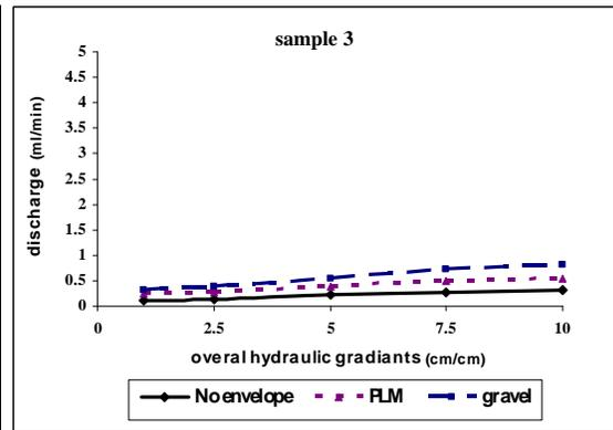
Figure 5. The variations of the outflow rate vs. the system hydraulic gradient.
