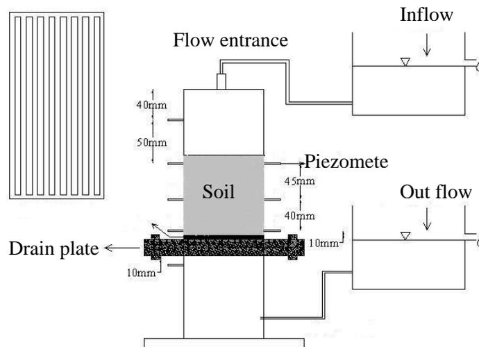
Figure 1. Schematic layout of one-dimensional downward flow permeameter in the laboratory
