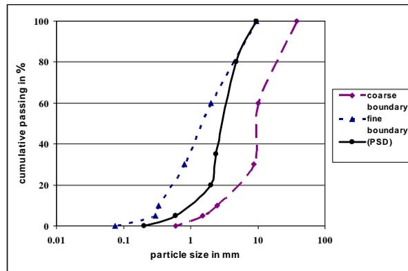
Figure 3. The mineral particle size distribution according to USBR standard.
