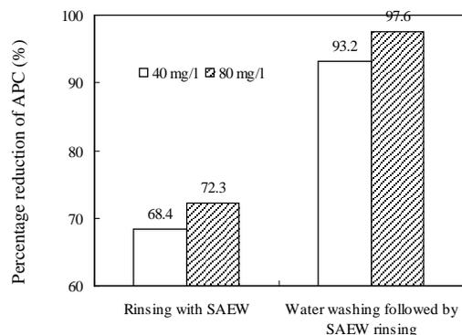
Figure 2. Disinfection effect of SAEW at ACC of 40 and 80 mg/l for milking cups.
