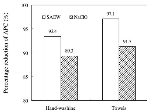
Figure 1. Comparison of disinfection efficiency between SAEW and NaClO solution at ACC of 20 mg/l for hand-washing and towels.
