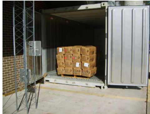
Figure 2. Pallet and antenna position during the readability study at an antenna distance of 2 m.
