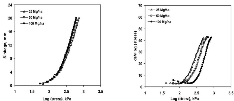
Figure 5. Sinkage ( $s$ ) and  $ds/d\log\sigma$  versus logarithm of vertical stress for plate sinkage test (PST). Results for soils amended with FYM with different application rates (25, 50, 100 Mg ha<sup>-1</sup>) at gravimetric water content of 20.9%
