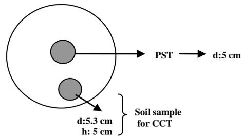
Figure 1. Top view of the large soil specimen and the locations of plate-sinkage test (PST) and soil sampling for confined compression test (CCT). d and h are the soil sample diameter and height, respectively.
