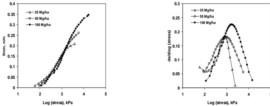
Figure 2. Strain ( $\epsilon$ ) and  $d\epsilon/d\log\sigma$  versus logarithm of vertical stress for confined compression test (CCT). Results for soils amended with farmyard manure (FYM) with different application rates (25, 50, 100 Mg ha<sup>-1</sup>) at gravimetric water content of 17.1%
