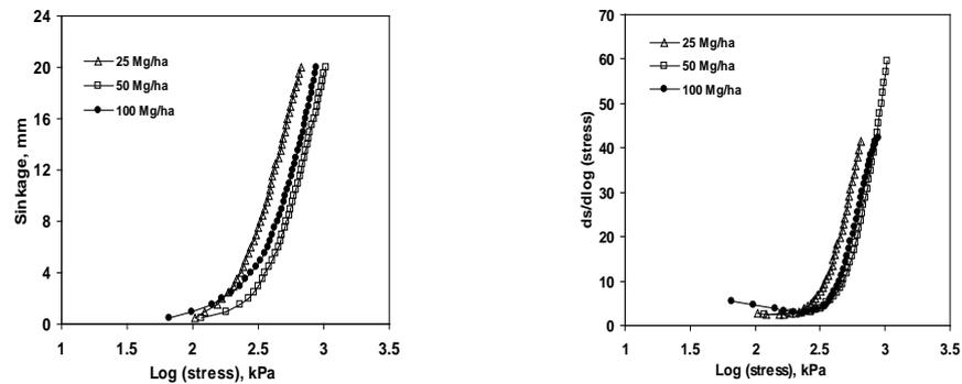
Figure 4. Sinkage ( $s$ ) and  $ds/d\log\sigma$  versus logarithm of vertical stress for plate sinkage test (PST). Results for soils amended with FYM with different application rates (25, 50, 100 Mg ha<sup>-1</sup>) at gravimetric water content of 17.1%
