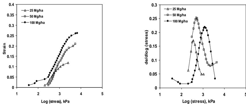
Figure 3. Strain ( $\epsilon$ ) and  $d\epsilon/d\log\sigma$  versus logarithm of vertical stress ( $\sigma$ ) for confined compression test (CCT). Results for soils amended with farmyard manure (FYM) with different application rates (25, 50, 100 Mg ha<sup>-1</sup>) at gravimetric water content of 20.9%
