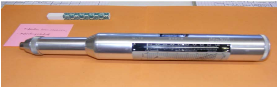
Figure 3. Rebound hammer, also named Schmidhammer.
