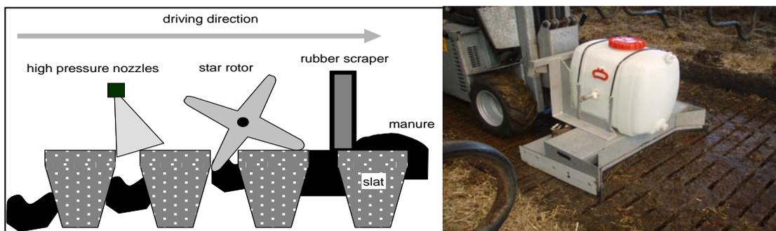
Figure 2. Plan of the different cleaning steps. Picture of the cleaning device with water tank
