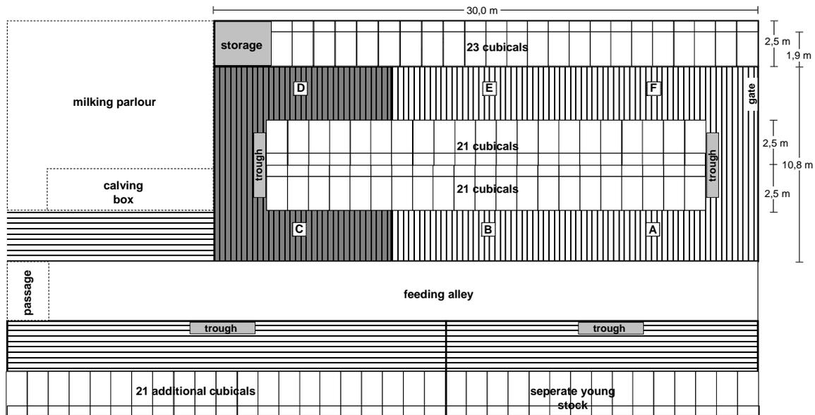
Figure 1. Floor plan of the barn. White vertical lining: cleaned experimental area. Grey vertical lining: control area in control treatment 2. Letters A-F: test elements. Horizontal lining: additional slatted floor, not included into the experiment.
