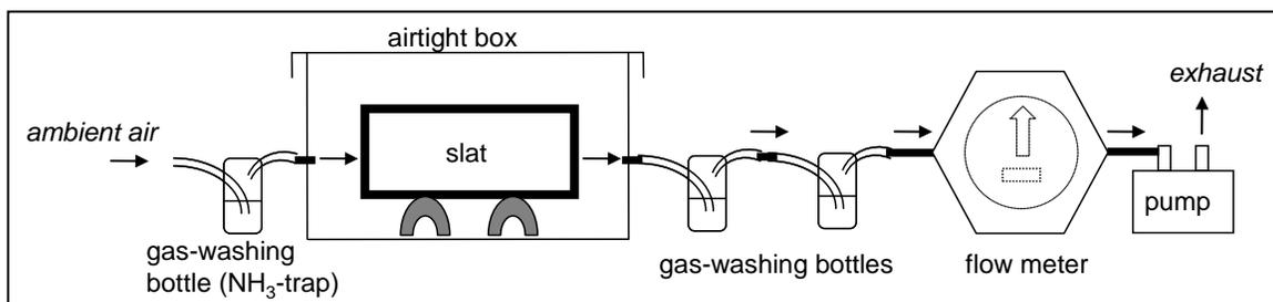
Figure 3. Set-up of one box and one slat element
