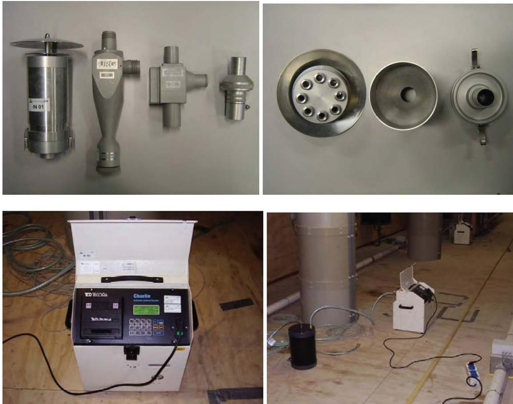
**Figure 1** Sampling equipment for PM<sub>10</sub> and PM<sub>2.5</sub>. Photograph upper left (from left to right): inlet, PM<sub>10</sub> and PM<sub>2.5</sub> cyclone collector and filter holder. Photograph upper right: adapted inlet for cyclone collectors. Photograph left bottom: the constant flow pump. Photograph right bottom: a constant flow pump connected to the condensed water collection vessel
