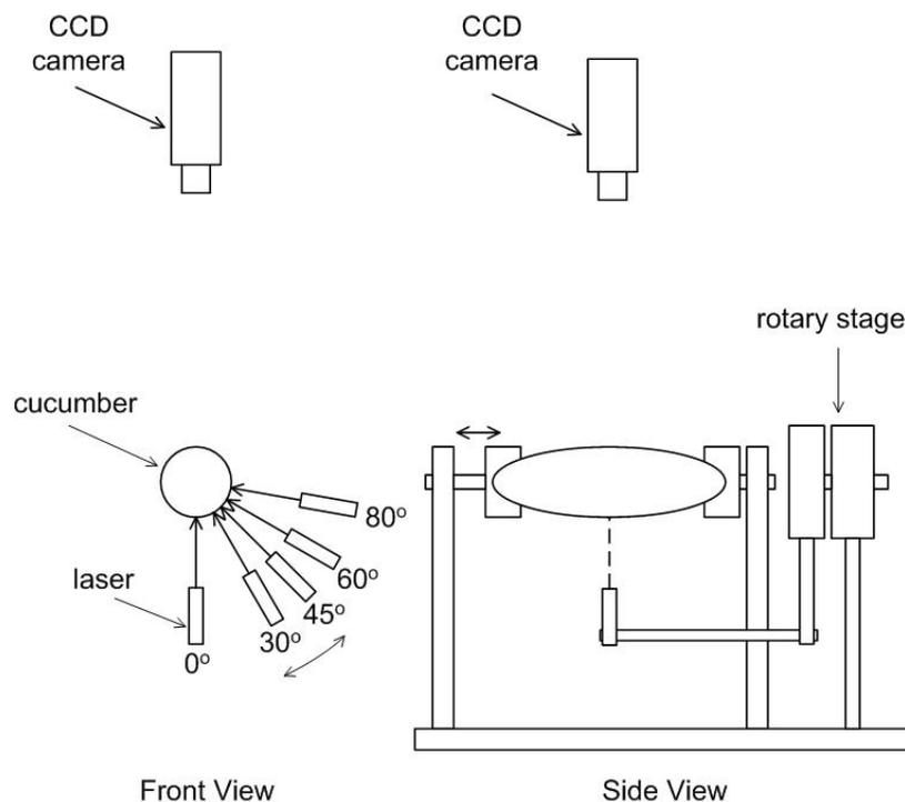
Figure 1. Schematic diagram of laser scattering experiment for detecting defective cucumbers.
