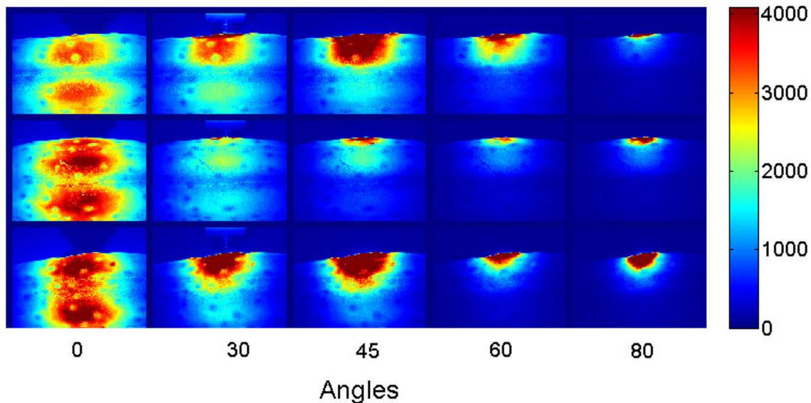
Figure 3. Laser scattering images at 0, 30, 45, 60, and 80 degrees of incident angle.
