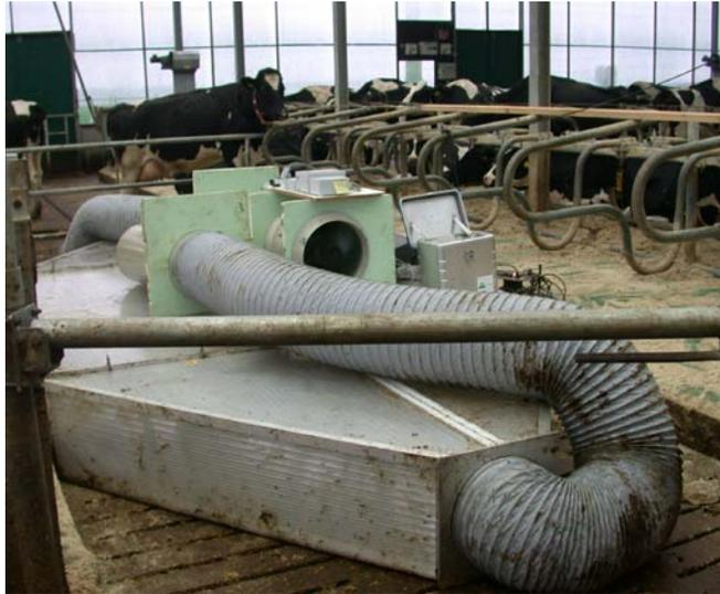
**Figure 1** Dynamic flux chamber.
