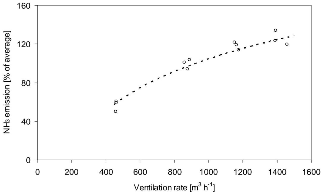
**Figure 3** Relation between the ammonia emission and the ventilation rate level of the ventilator in the chamber
