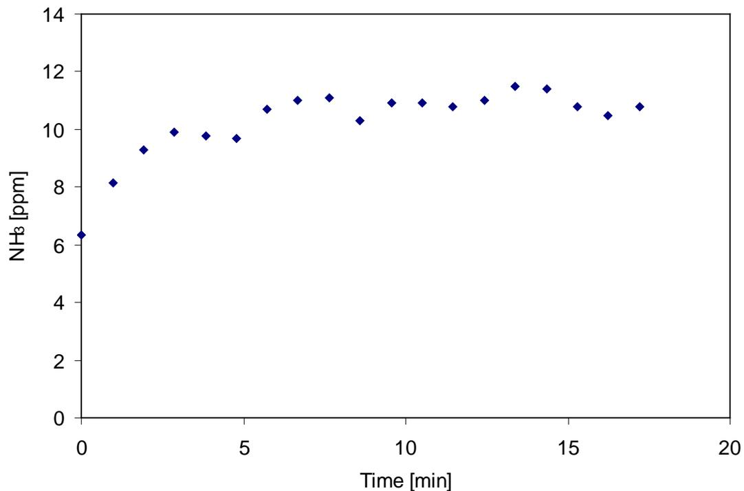
**Figure 2** Ammonia concentration pattern inside the dynamic flux chamber. Applied
