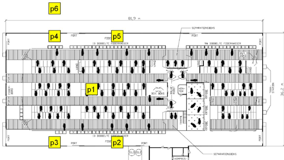
Figure. 1. Measurement section and sensor positions
