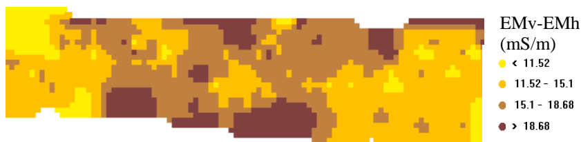
Figure 2 A raster map of the difference between EMv and EMh measurements
