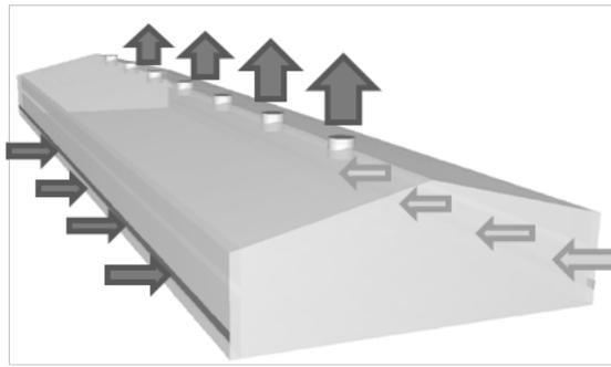
(a) case1 – side wall in, roof out
