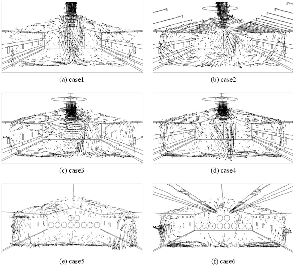
Figure 4. Air velocity vectors in the broiler houses.
