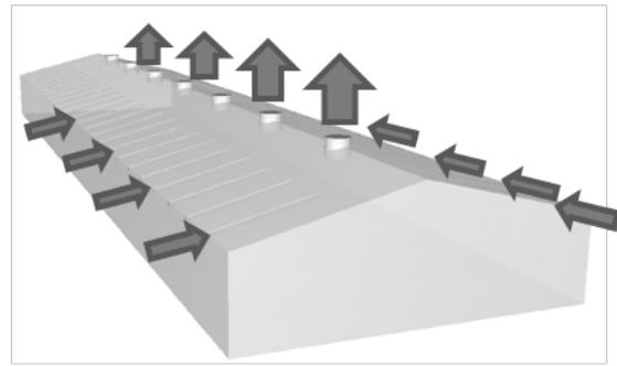
(b) case2 – pipe in, roof out
