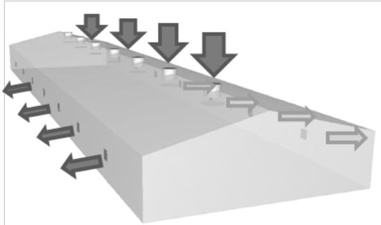
(c) case3 – roof with diffuser in, side out
