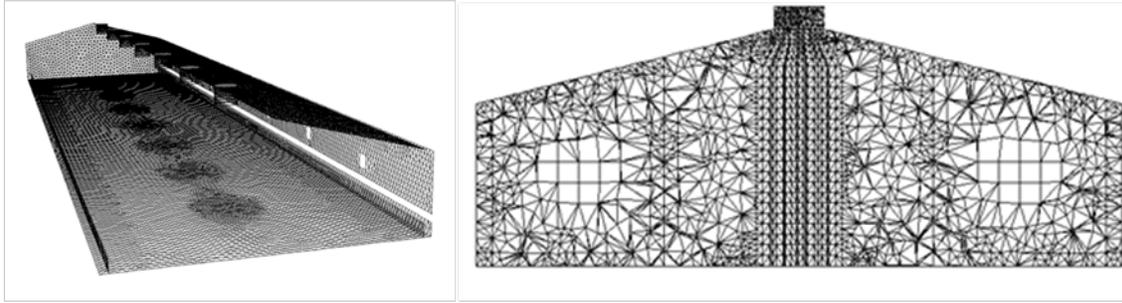
Figure 2. Constructed geometry and mesh design of case 1 using GAMBIT
