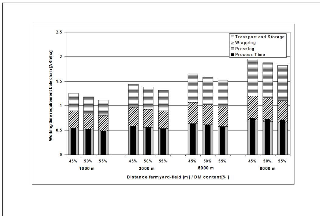
Figure 3. Working time requirement and process time for the square bale method in dependence on the field-to-farm distance and the dry matter content.
