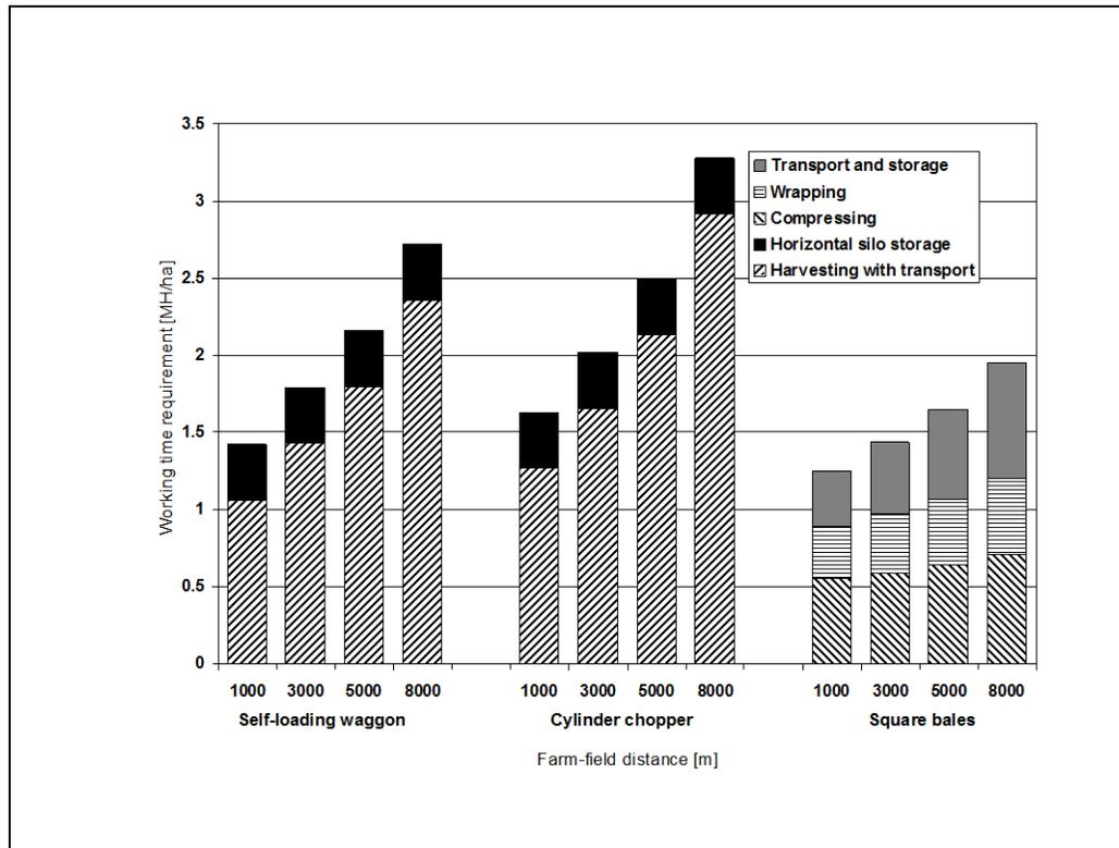
Figure 4 Working time requirement of different process chains for the harvesting of grass silage, dependent on field-to-farm distance.
