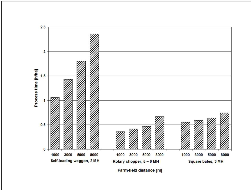
Figure 5. Process times of different harvesting chains for grass silage, dependent on field-to-farm distance.
