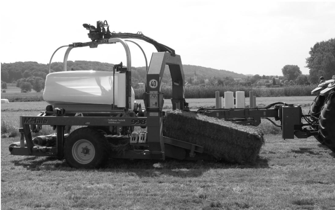
Figure 2. A second bale can be picked up while one bale is still being wrapped. This considerably increases equipment efficiency.
