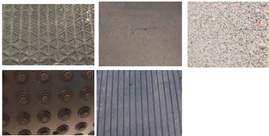
Figure 2. Top and bottom view of three tested materials: on the left, rubber mat with burls; in the middle, mat with grooved bottom side; on the right the resin coat.
