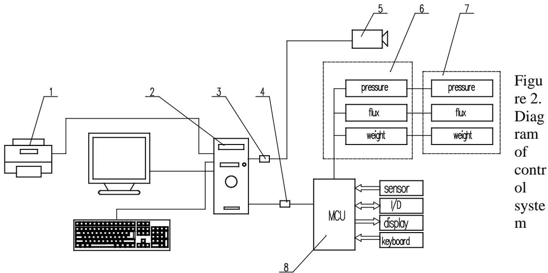
Figure 2. Diagram of control system
