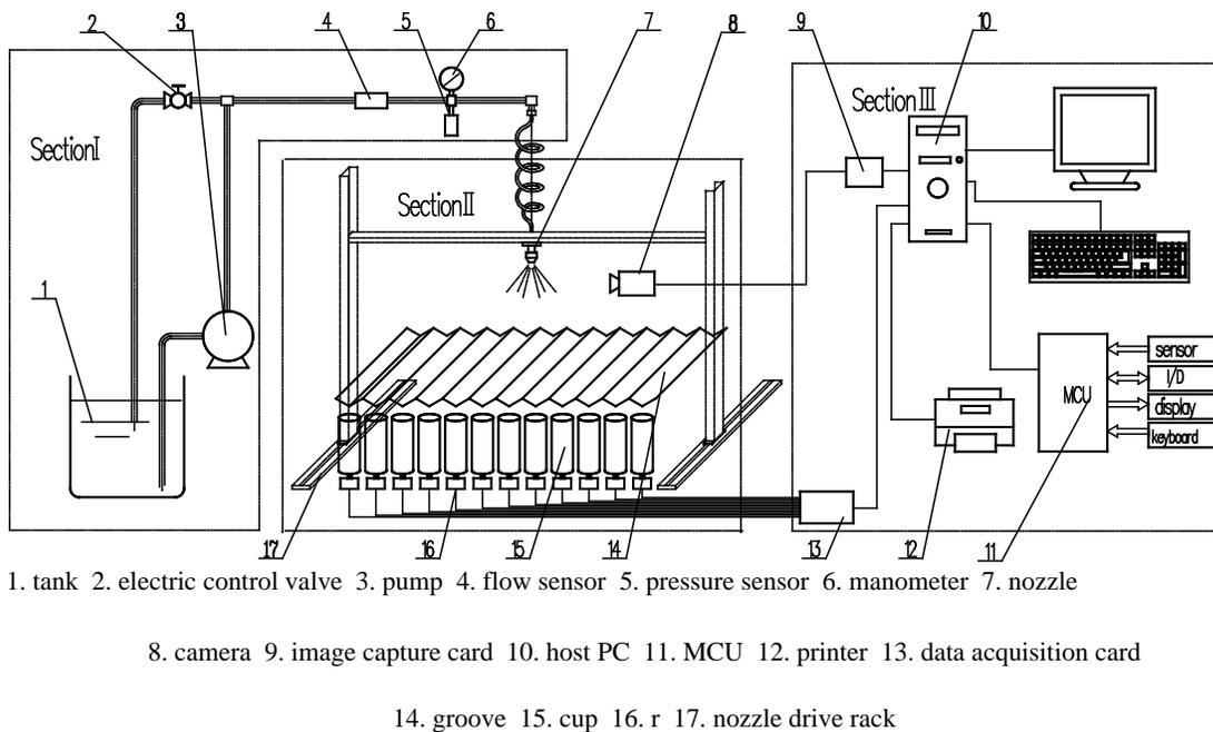
Figure. 1 Diagram of the distribution system
