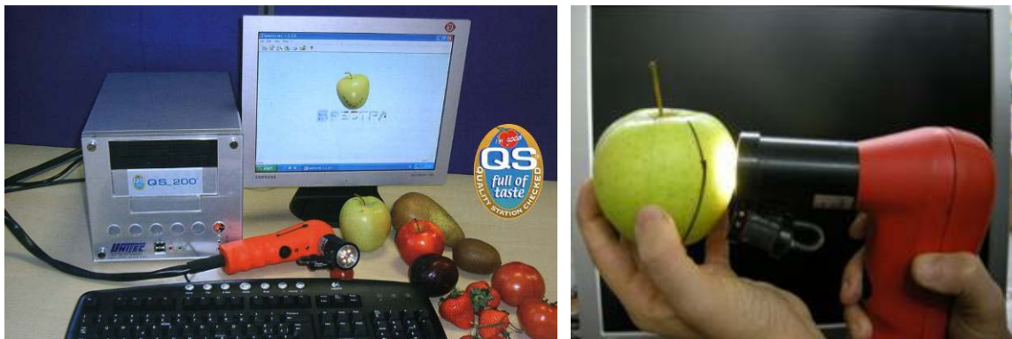
Figure 1 – Image of QS_200 desk system and particular of spectral acquisition process
