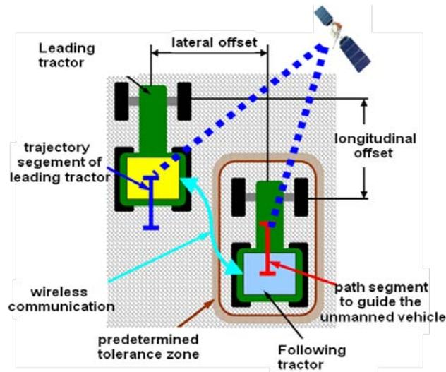
Figure 2. Schematic diagram of the towing bar system for two tractors using GPS navigation and wireless data exchange
