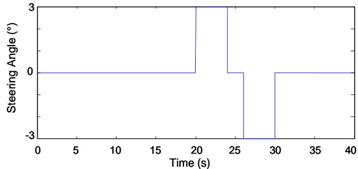
Figure 8: Steering angle change of the leading vehicle
