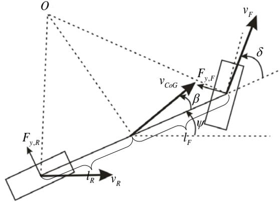
Figure 6 Dynamic Model of the Unmanned Vehicle
