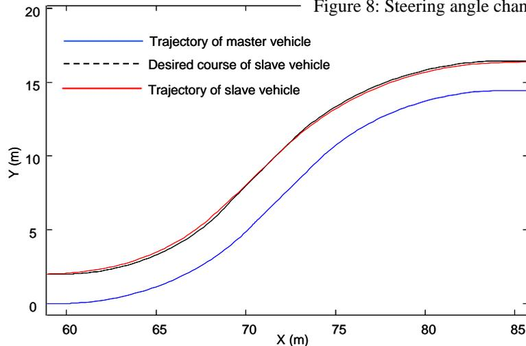
Figure 9: Simulation result of the tracking control (20s~30s)
