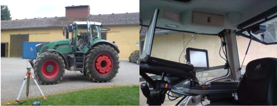
Figure 1. Fendt 936 Vario tractor and its cabin with machine guidance terminal
