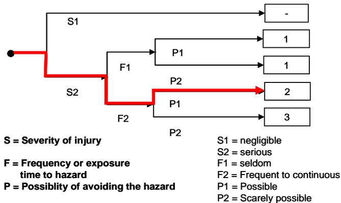
Figure 11: Classification of safety-related system in different safety-integrity-level according to IEC 61508
