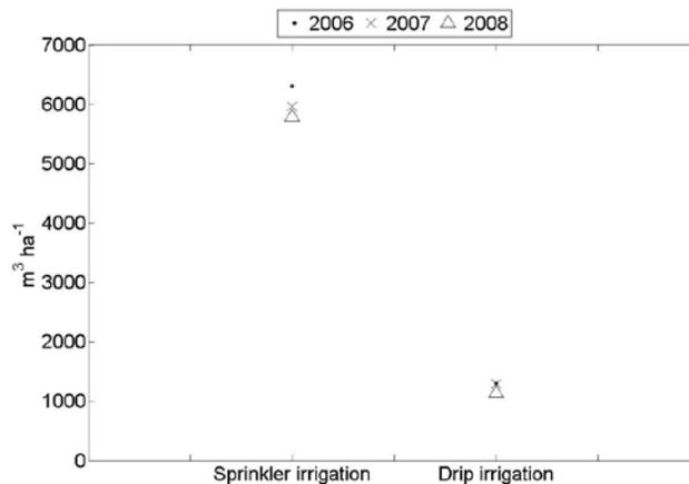
Figure 1. Annual irrigation water supply per unit irrigated area ( $V_{TSr}$ ,  $m^3 ha^{-1}$ )
