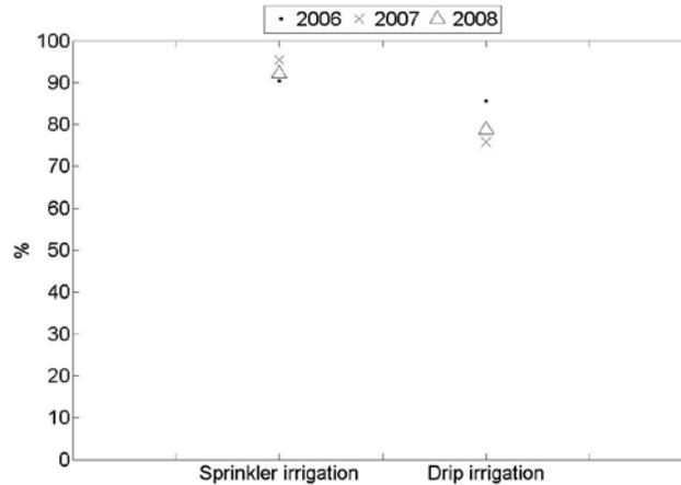
Figure 2. Main system water delivery efficiency (ED, %)
