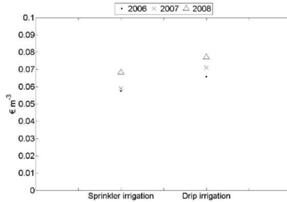
Figure 3. Energy cost per unit irrigation delivery (CENVs, €m<sup>-3</sup>)
