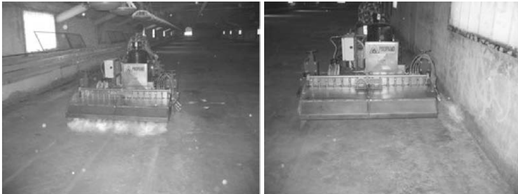
Figure 2. Flaming treatment in broiler house.
