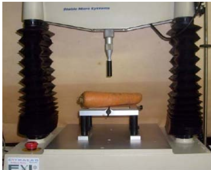
Figure 1. Illustration of the penetration test.
