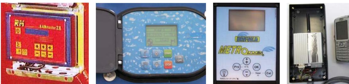
Figure 6. Control units and modem GSM for remote control.
