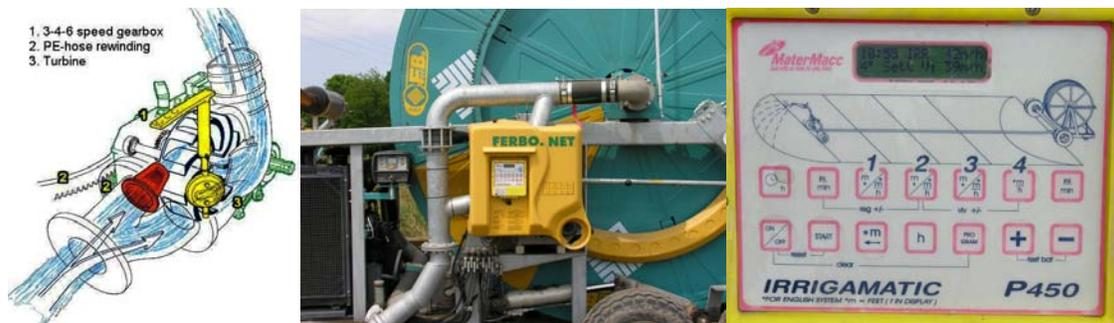
Figure 9. Automated variable transmission. Turbine is fastened on the driving gear shaft.
