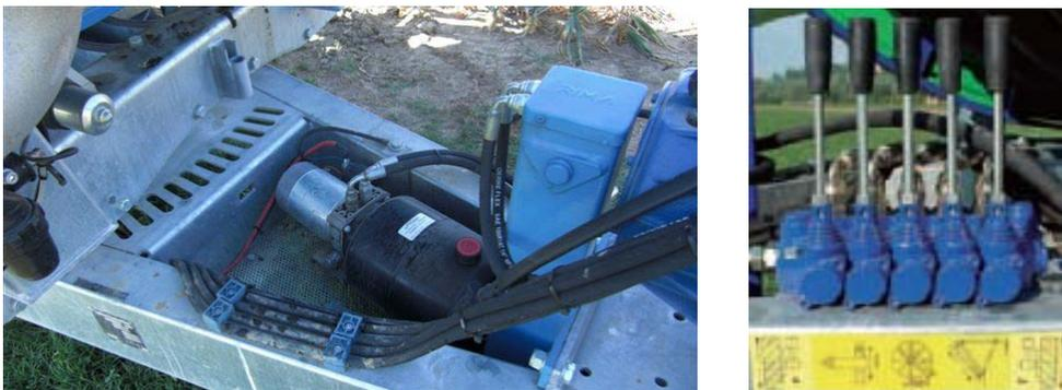
Figure 2. Pipes and control sticks of the hydraulic devices.
