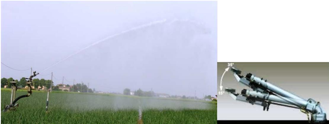
Figure 5. Jet atomization (left) and sprinkler with variable jet angle (right).
