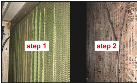
Figure 2. Experimental setup 2 consisting of two filter elements. A cellulose filter element with 40 % larger volume specific surface area than traditional cellulose filters and a biofilter consisting of 30 cm crushed tree roots.
