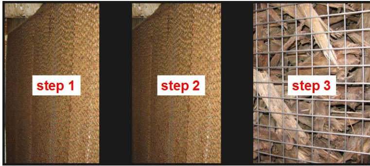
Figure 1. Experimental setup 1 consisting of three filter elements. A Farm AirClean BIO module extended with a biofilter consisting of 60 cm thick layer of crushed roots.
