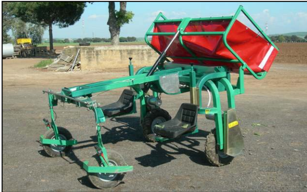
Figure 3. General view of the zucchini harvester arranged for harvesting artichoke.
