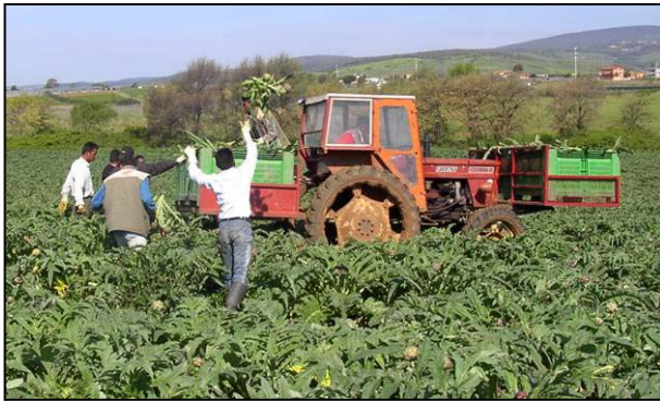
Figure 2. “Over the row” tractor with rear and front frames to hold bins.
