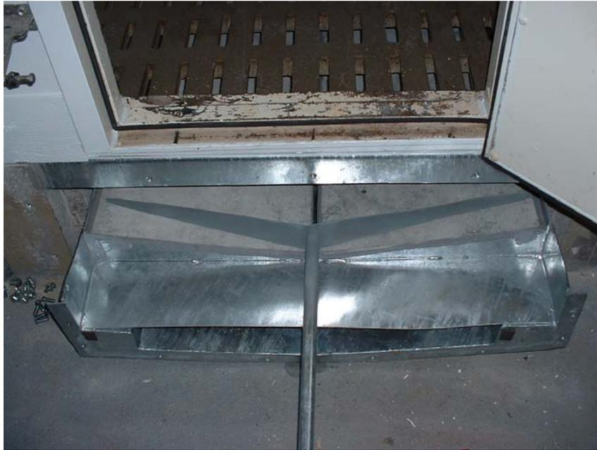
Figure 2. A picture of the V-shape scraper system.
