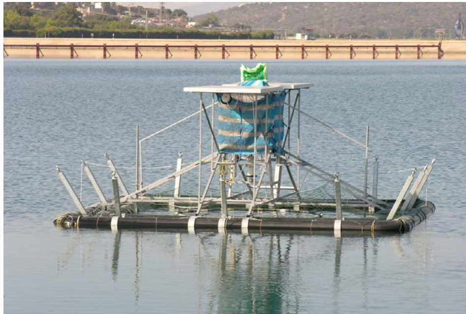
Figure 4. The fishing machine used as a part of the "Virtual-Cage culture". It enables scheduled fish training and periodic re-training. It traps fish by 'calling' them to feed and automatically closing a net which hangs underneath it by lifting its fringes above water level.
