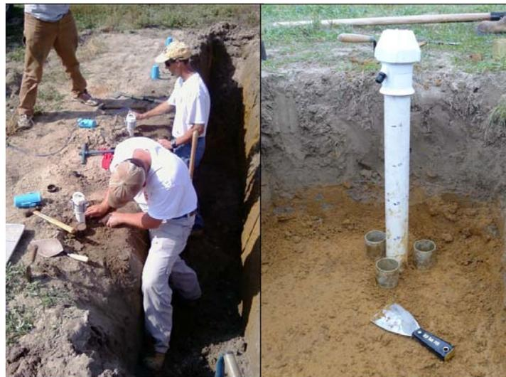
Figure 2. Calibration trench and ring sampling technique.
