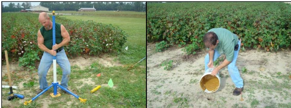
Figure 1. Probe installation techniques: Direct (left) and Slurry (right)
