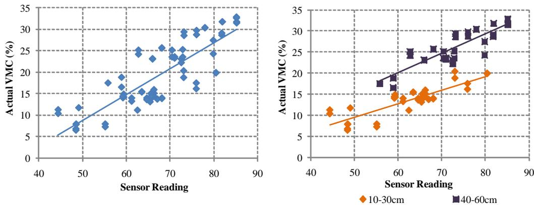
Figure 5. VMC vs. the AquaSpy sensor readings for all data (left) and horizon separation (right).
