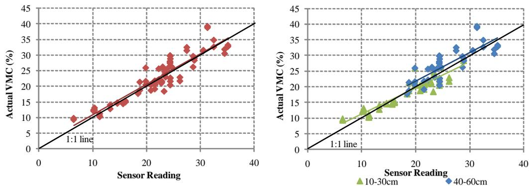
Figure 4. VMC vs. the Sentek sensor readings for all data (left) and two different horizons (right).
