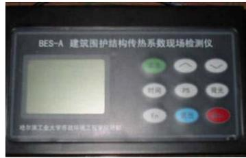
Figure 2 Overall Heat Transfer Coefficient of Building Envelope Detector
