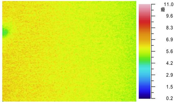
Figure 10 average temperature of the north side wall of the north side room 5.87 °C wall
