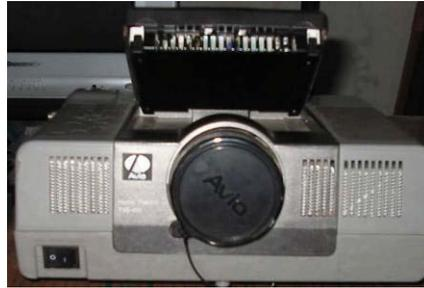
Figure 3 Portable Thermal Infrared Imager
