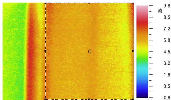
Figure 8 average temperature of the north side wall of the north side room  $5.65^{\circ}\text{C}$
