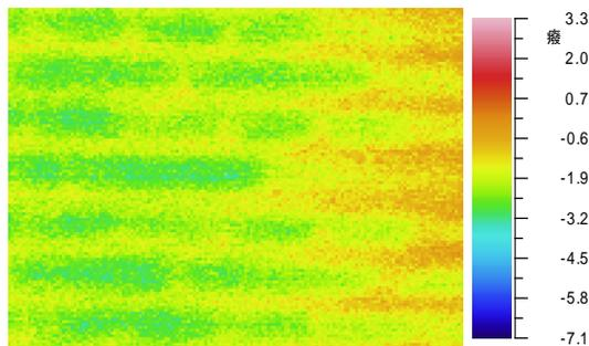
Figure 9 average temperature of the east side outside wall of the north side room  $-1.83^{\circ}\text{C}$
