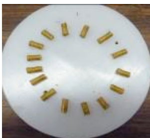
Figure 2. Pellets produced from the pretreated biomass using single pelleting Instron machine.
