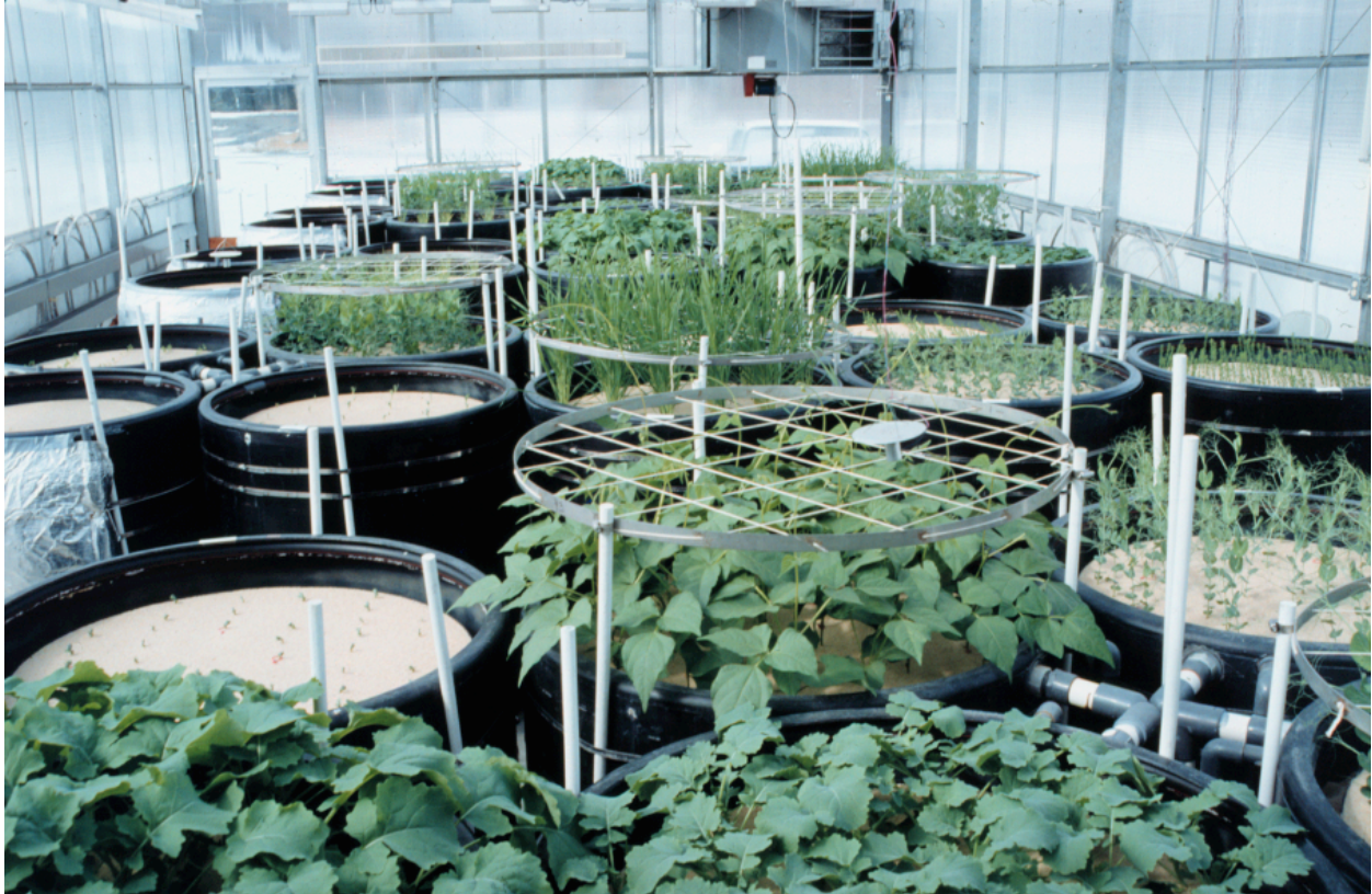
Figure 3. Canada's "SaltLab" houses a field-simulating, environmentally-controlled testing facility to measure the response of Canadian crops to root-zone salinity.
