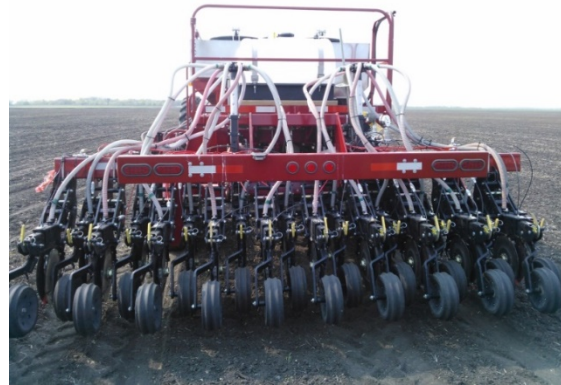
Figure 2. Salford 522 air drill.
