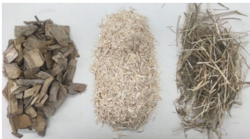
Figure 1. Raw biomass used for microwave pyrolysis experiments (right to left: maple hardwood, spruce softwood, and switchgrass).
