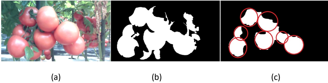
Figure 6.(a)Tomato skewers containing multiple tomato fruits,(b)Tomato skewers binarized image,(c)Multi-target fruit recognition based on Hough transform.
