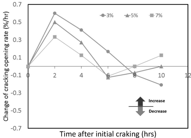
Figure 6. Changes of crack opening rate for mixtures with various fibrous agro-waste contents
