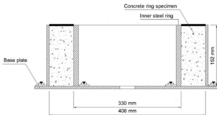
Figure 2. Ring test to evaluate cracking time and increase in crack width
