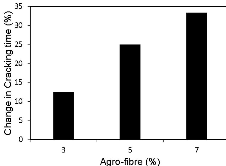
Figure 4. Changes in cracking time at various fibrous agro-waste contents
