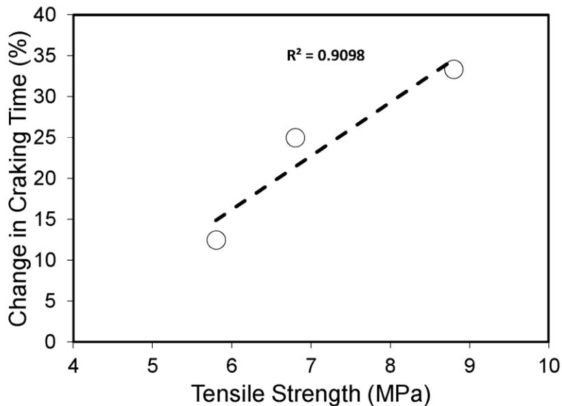
Figure 5. Correlation between changes in cracking time and tensile strength for mixtures with various fibrous agro-waste contents
