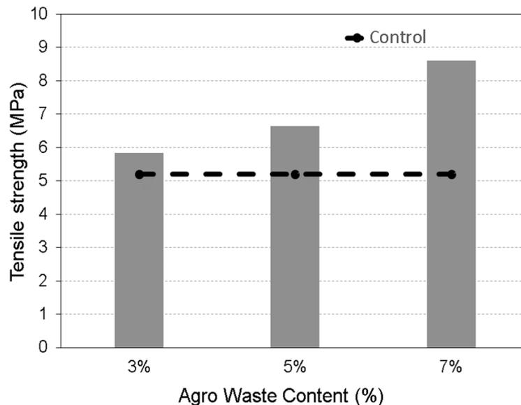
Figure 3. Tensile strength results for mixtures with different fibrous-agro-waste contents
