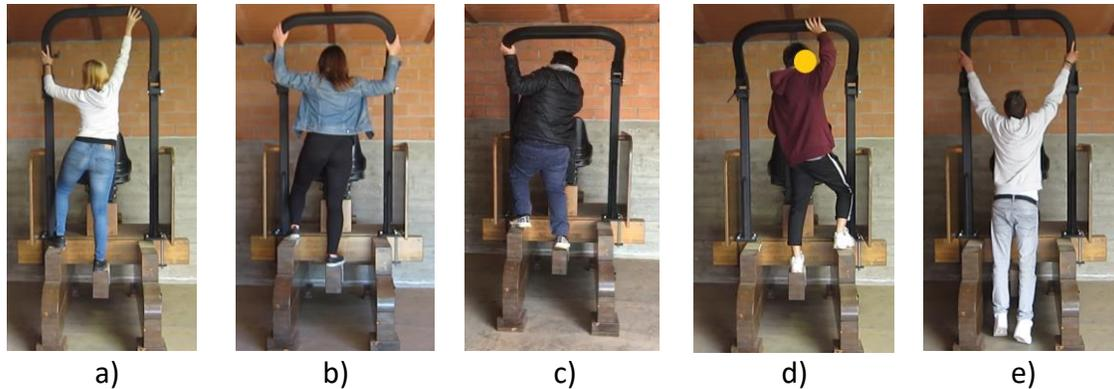
Figure 2. Participants while raising the traditional FROPS: the shortest (a) and the tallest (b) female participants, the shortest male participant (c), the tallest male participants using parts of the structure as a support for the feet (d), and maintaining his feet on the ground (e).
