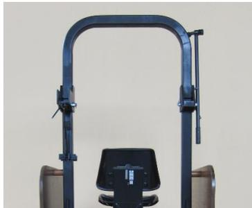
Figure 1. The prototype of the supporting devices fixed on the FROPS. On the right side the rod, and on the left side the gas spring were welded.
