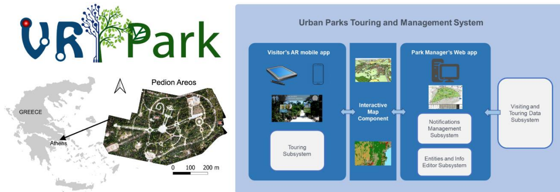
Figure 1. The pilot park of the “VR-Park” project and the general structure of the overall proposed touring system.
