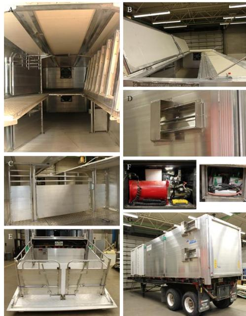
Figure 1. Photos of the animal compartment showing (A) its lower and upper decks, (B) hinged roof, (C) gate that partitions each deck into two pens, (D) air exhaust damper, (E) hydraulic lift gate, (F) hydraulic lift controller and (G) compartment exterior.
