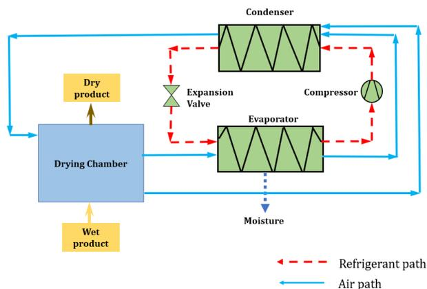
Figure 1. Schematic diagram of heat pump dryer.
