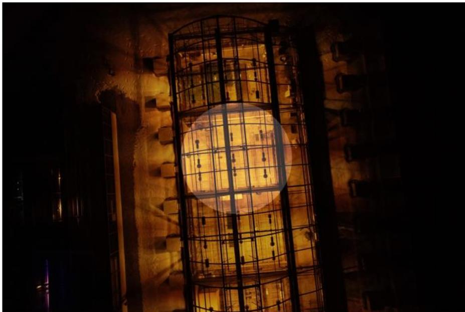
Figure 2. Representation of the analyzed area of the camera images which match the FOV (field of view) of the SQM. The lighter shaded circle in the center is the portion of the camera image that was analyzed for intensity values.
