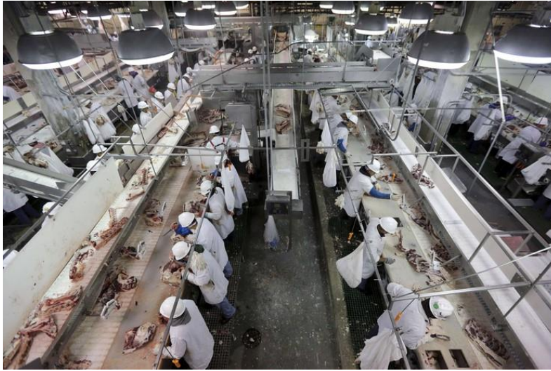
Figure 1. Workers employed at Cargill beef processing plant cut excess fat and meat off primal cuts (i.e. ribs, tenderloin, etc.) in order to fit specification. The leftover trim is gathered on a separate conveyer belt. Employees wear plastic sleeves and gloves in order to minimize
